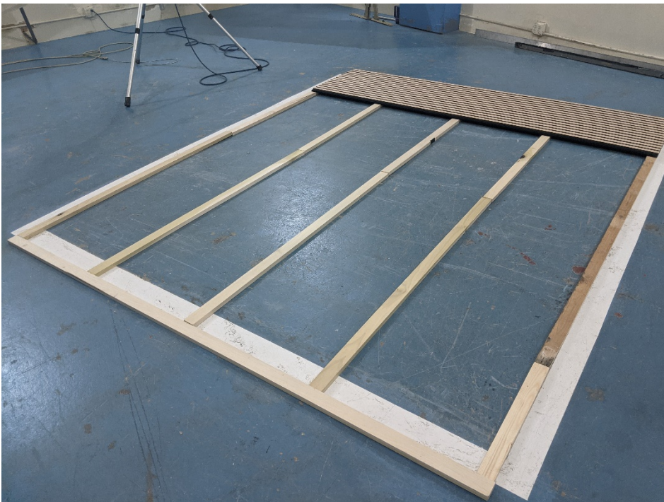
Figure 2 – Specimen partially installed over spaced furring strips
